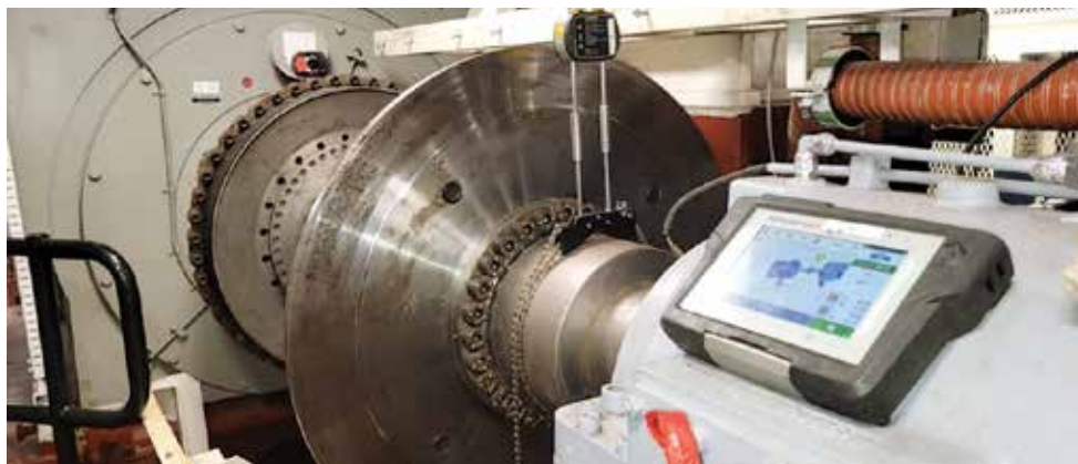
A laser (the two mounted gauges above the shaft) send alignment info to the analyzer.
