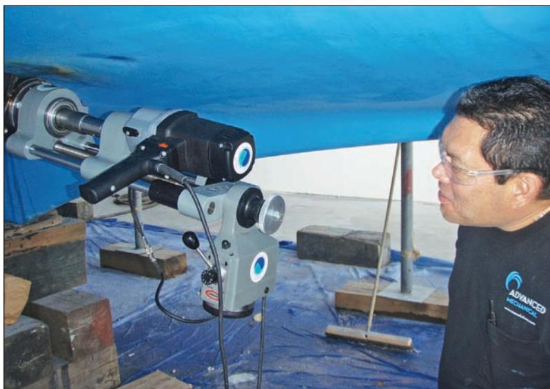
When a Donzi Yachts client wanted his sportfisherman retrofitted with the BOSS shaft and thrust bearing assembly, the builder retained Advanced Mechanical Enterprises to precisely increase the diameter of the stern-tube bore.
