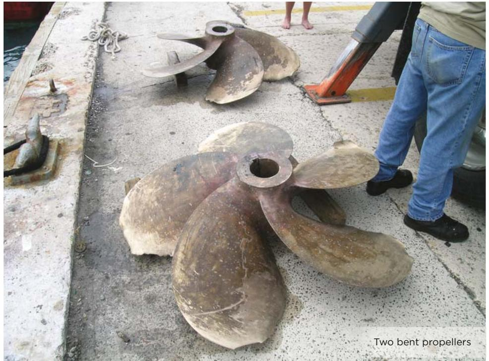
Two bent propellers
