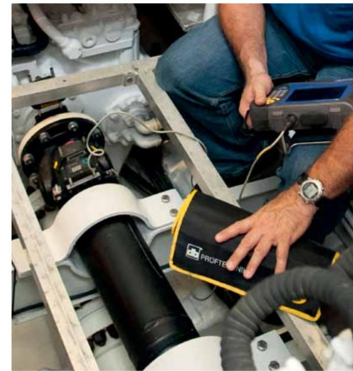
Checks are made for machinery vibration being transmitted through the hull (left), and the Rotalign Ultra unit is fitted to a Cardan shaft (above)
