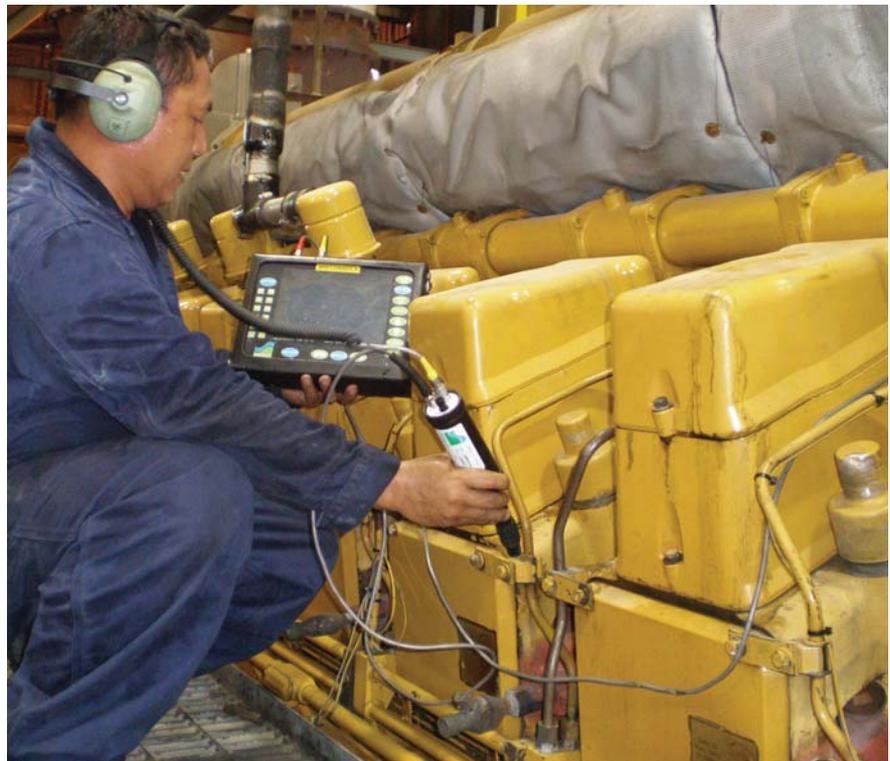
Sales, Windrock. “auto-balancing” of cylinder firing pressures with the patented Windrock AutoBalance™ system on larger natural gas engines has been successfully used to control emissions, reduce fuel costs and reduce the overall mechanical degradation of mechanical components due to imbalances.”
