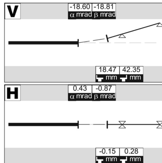
The Rotalign Ultra computer displays a machinery graphic (above), while the result of the final laser alignment of the Cardan shafts in the horizontal and vertical planes is shown in the graphic on the left
